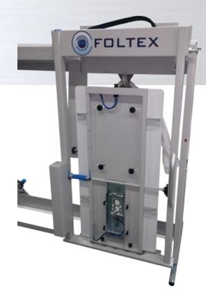
Once the bathrobe is horizontal and the front of the garment is facing down, the operator can manually fold the sleeves so that mechanical blades can create the primary folds and cross fold.
