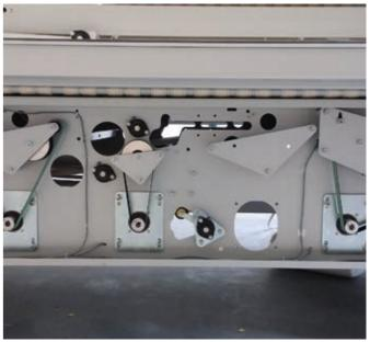
and the third cross folds are made by reversing belts in combination with a knife. Both light as well as thick items can be processed against highest folding quality. By means of automatic wide measurement it is possible to bypass the third cross fold for small items, while it is enabled for large items.
