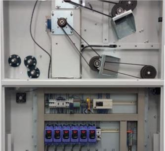
maintenance-free photocells (no reflectors). The FlexFold LP300-400 is a machine built for life and requires little maintenance in comparison with competing folders. The drive system of the lateral fold section is done by maintenance-free timing belts.
