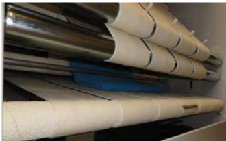
reversing belts. Tight folded pieces are obtained as pieces are continuously kept between belts. The elastic belts ensure that the cross fold automatically adapts on thin as well as thick pieces. Pieces are supported over the full width of the 2nd cross fold, eliminating the chance of jams.
