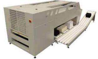
out over the stacker stations. Once the required stack height is achieved, the stack is put on the final delivery belt. The stack is brought onto the final incline belt by means of a slide mechanism ensuring a smooth and straight transfer.
