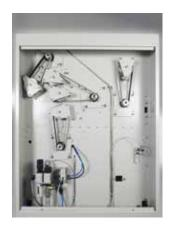
retracted. The retracting movement is carried out by 2 oversized cylinders and controlled by an intelligent linear encoder. This way the movement is carefully monitored and controlled, ensuring a long operating lifespan.
