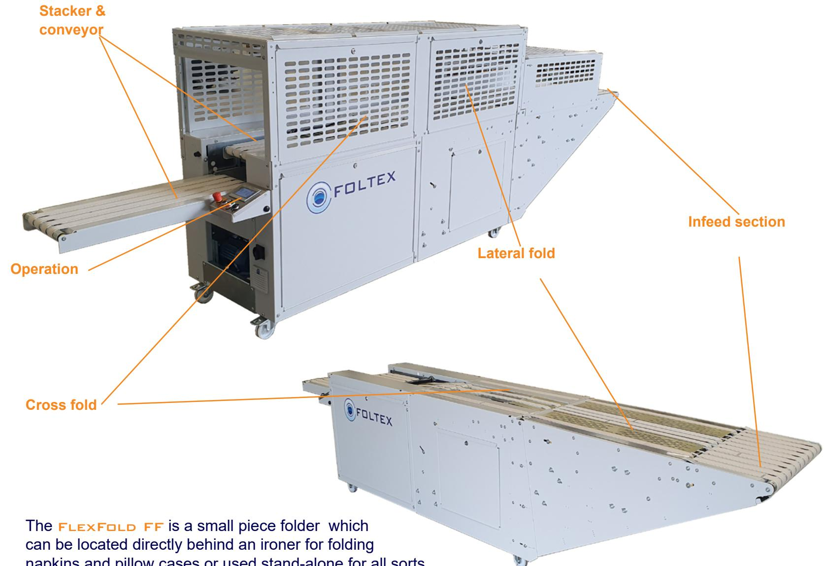
The **FLEXFOLD FF** is a small piece folder which can be located directly behind an ironer for folding napkins and pillow cases or used stand-alone for all sorts of dried linen and garments. The FlexFold FF is the answer when accurate folding is required.
